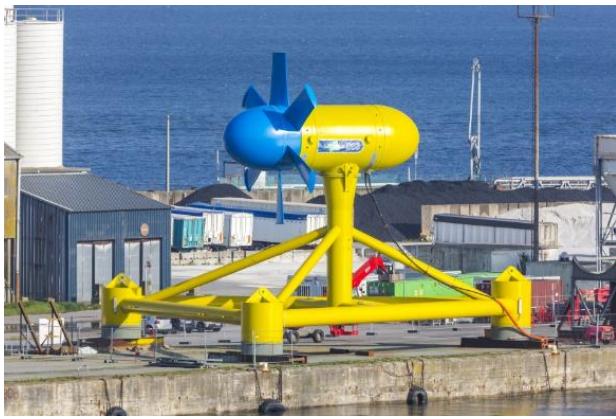
Fig. 3. Image of the Sabella D10 rotor on dockside.
