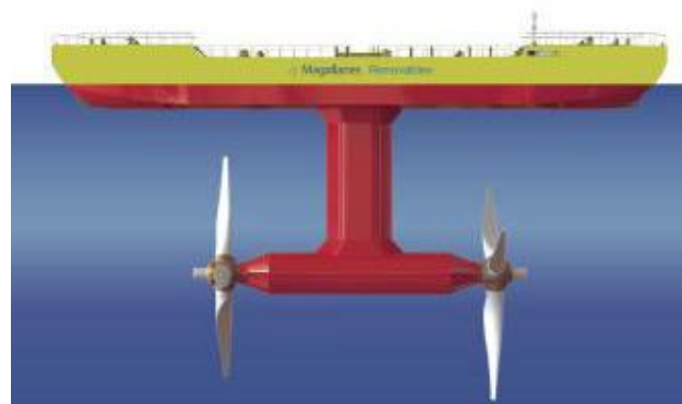
Fig. 2. Schematic side view of the Magallanes ATIR rotor.
