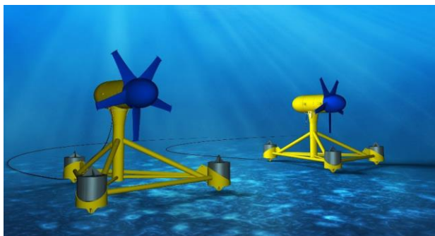
Fig. 4. Proposed design of the Sabella D12 rotor in small array configuration.
