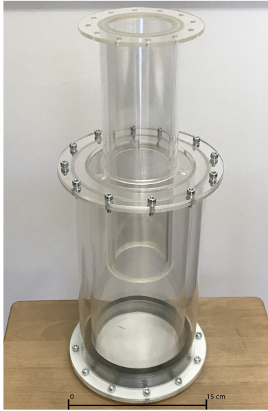
Fig. 2. Physical model used in experiments (1:100th scale).
