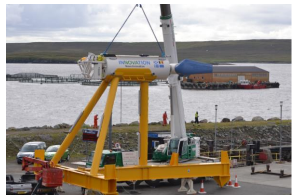
Fig. 4. Nova Innovation tidal turbine M100 bi-directional turbine with 100kW rated capacity.
