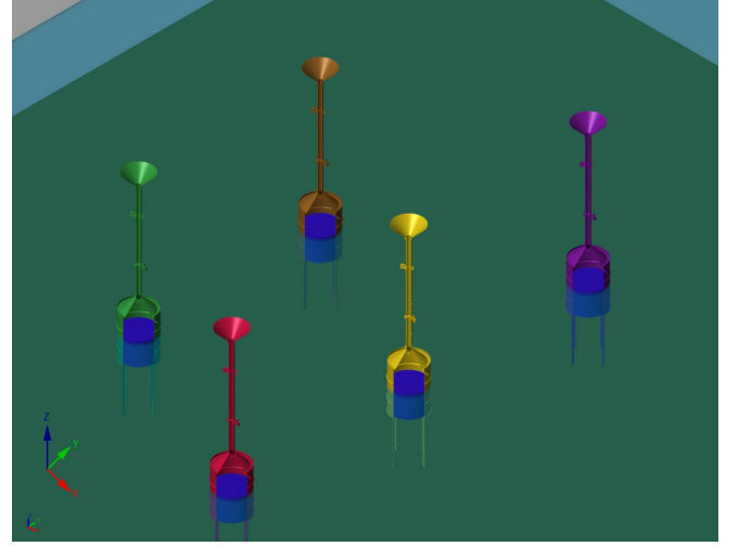
Fig. 3. WEC-Sim Non-optimal array layout. Blue cylinders are hydrodynamic bodies. Multi-colored bodies are for visualization only.
