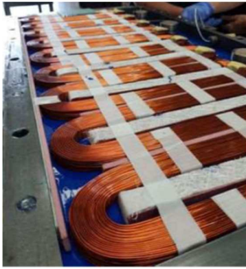
Fig. 11. Assembly of nine coils for potting into an epoxy coil blade
