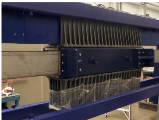
Fig. 8. Single complete translator installed on a single generator/motor stator assembly in the horizontal position prior to being raised into the vertical position. Stator assembly indicated top and bottom of translator
