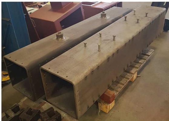
Fig. 7. Translator central support structure pre-fabrication
