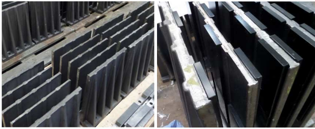
Fig. 5. Magnet modules. Left: Cast magnet modules ready for magnet insertion. Right: Magnet module with magnet insertion underway
