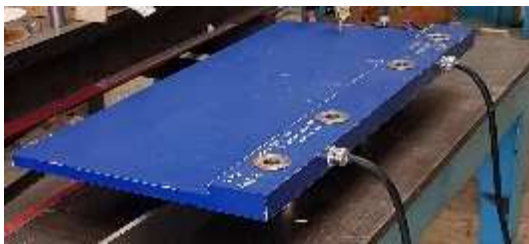
Fig. 13. Completed epoxy potted coil blade
