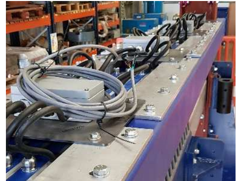
Fig. 15. Wiring of motor coil modules in horizontal position
