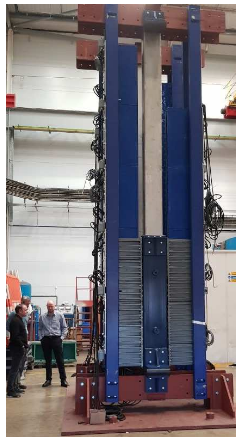
Fig. 16. C-GEN Project Neptune test rig, motors and generators in vertical position ready for counter balance installation
