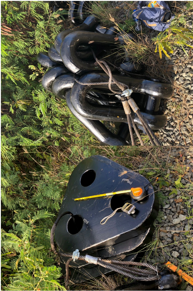
Fig. 9a. WETS 60m berth mooring components, including (top) 102mm D-shackles used beneath the surface float and as joining links between shots of chain, and (bottom) tri-plates which join surface float chains to main chain and WEC or no-WEC hawser systems.
