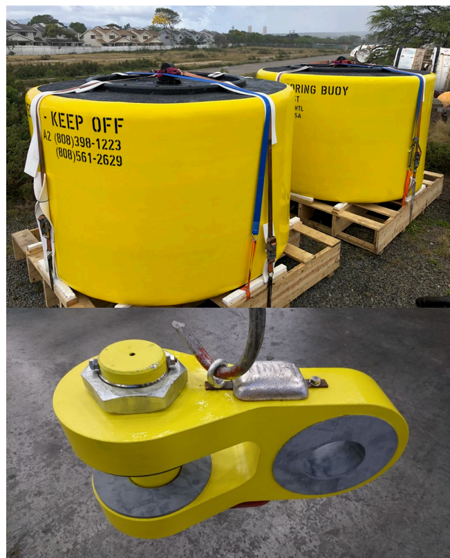
Fig. 11. WETS 60m berth mooring components, including (top) surface floats and (bottom) a representative U-link, which is attached to the buoy padeye and to a 102mm D-shackle (as shown in Fig. 10).
