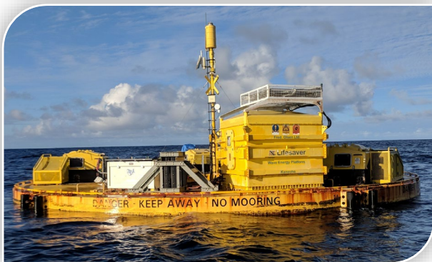
Fig. 5. Fred. Olsen Lifesaver with Wave Adaptable Monitoring Package (WAMP) installed. WAMP is in lowered (operational) position, with support structure to right of white electronics housing.
