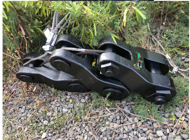
Fig. 9a. WETS 60m berth mooring components, including (top) 102mm D-shackles used beneath the surface float and as joining links between shots of chain, and (bottom) tri-plates which join surface float chains to main chain and WEC or no-WEC hawser systems.
