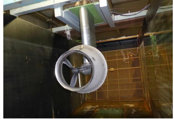
Fig. 9. Experimental setup of the optimized turbine with the shroud in the circulating water channel.
