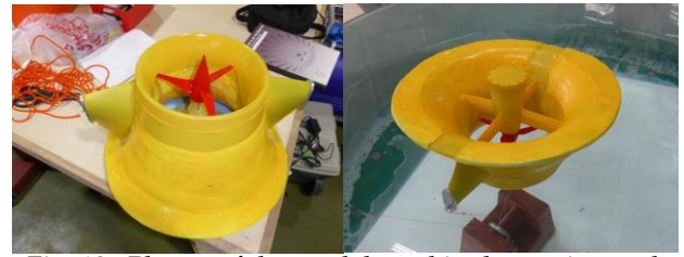
Fig. 13. Photos of the model used in the towing tank experiments.
