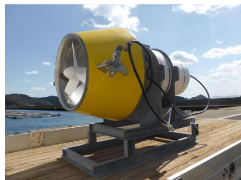
Fig. 17. A photo of the floating/submersible shrouded tidal current turbine for the demonstration experiment in the Naru Strait in Goto, Nagasaki.
