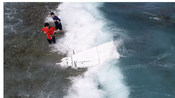
Fig. 19. Ducted-WEC concept, and 1st prototype model made by aluminum plate. We attached the half scale WEC to the end of this taper.
