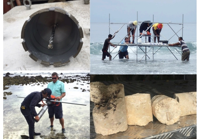
Fig. 4. Drilling into the sea floor with core drill. We used a gasoline engine (75 cc cylinder two-cycle) to drive the core drill.
