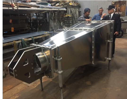
Fig. 19. Ducted-WEC concept, and 1st prototype model made by aluminum plate. We attached the half scale WEC to the end of this taper.
