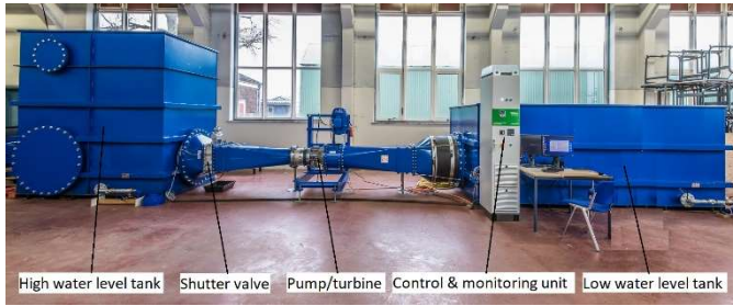
Fig. 2 Climate Power Plant Simulator, laboratory HZ University of Applied Sciences.
