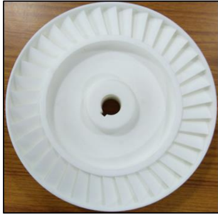
Fig.4. 3D printed rotor
