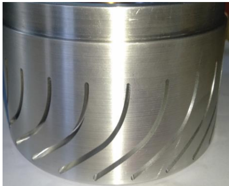
Fig. 5. Groves cut in the hub
