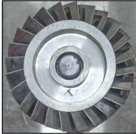
Fig.3. Fabricated guide vane
