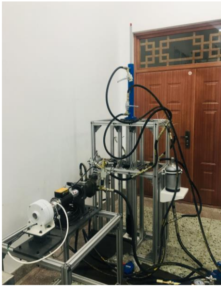
Fig. 25. Hydraulic PTO test bench
