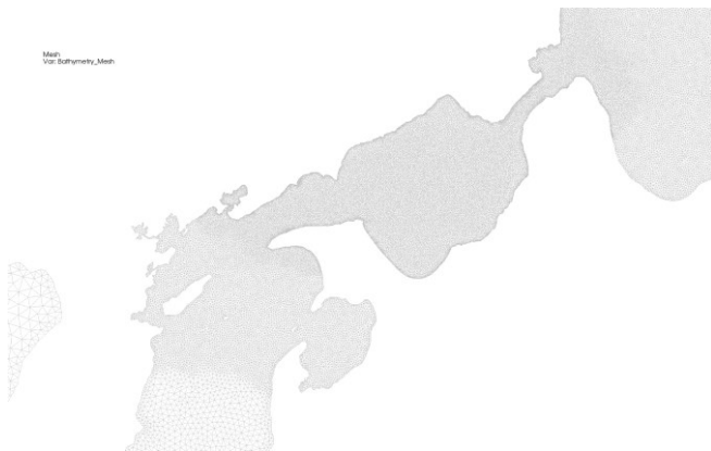
Fig. 5. Zoom-in view of the numerical model grid in the narrows region of the strait, with a grid resolution of up to 100 m.
