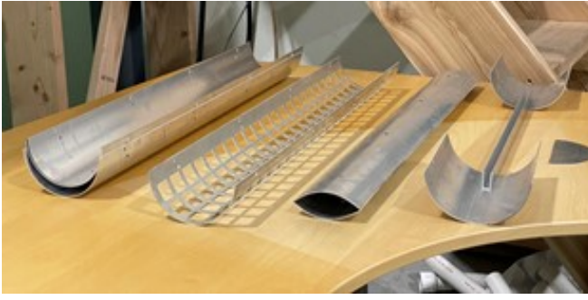
Fig. 9. Reaction plate test articles laser cut from aluminum
