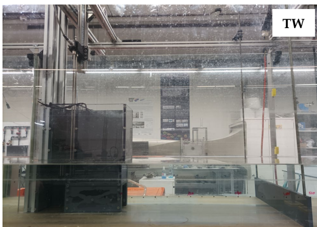
Fig. 6. Transversal wall (TW) of 80 mm installed in front of the model representing the Mutriku power plant.
