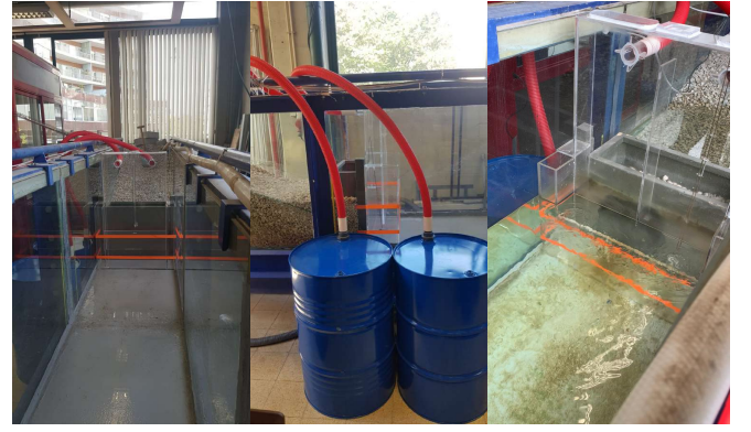
Fig. 2. Views of the U-OWC model installed at the IST wave flume. The blue barrels in the photos were used to simulate the effects of air compressibility.
