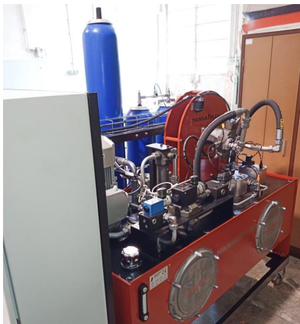
Fig. 10. Oil-hydraulic HIL test rig for testing the hybrid and active accumulator PTO concept (Grant contract PTDC/EME-REN/29044/2017).
