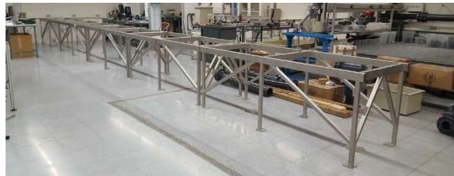
Fig. 2. Main lower structure: One module CAD (Top) and five modules in mounting process (Bottom).
