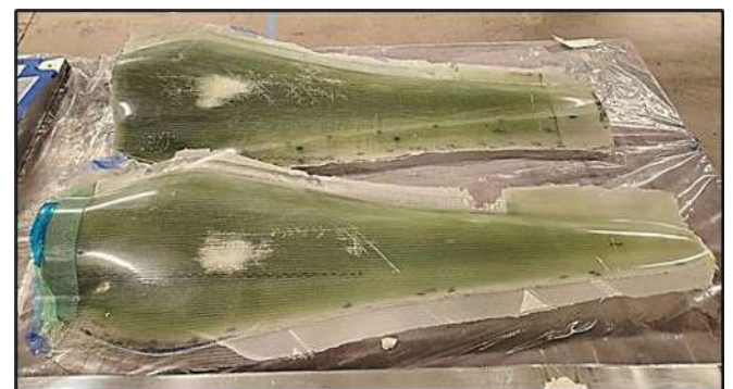
Fig. 15. Composite blade skins.
