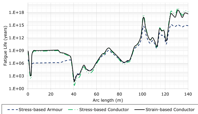
Fig. 9. Original model: fatigue life in years of the power cable considering the different segments and cable components.
