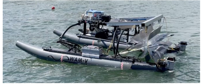
Fig. 8 Assembled MHK platform as of March 2023
