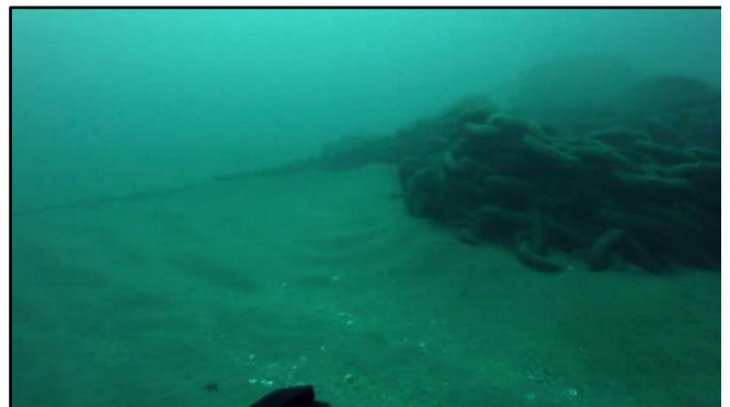
Fig. 12. Sand accumulation in the western side of one of the chain weights, at BiMEP.
