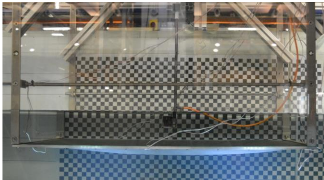
Fig. 1. Photograph of the flexible neoprene rubber material arranged inside the wave flume supported by four flat rods at the edges.
