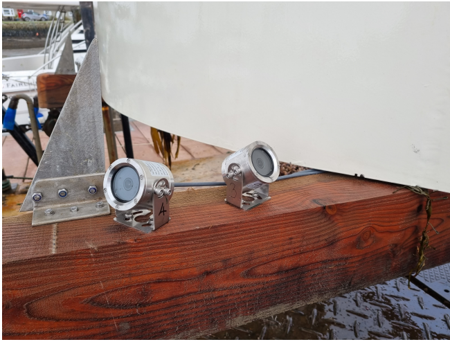
Fig. 4. The port side cameras with the rotor facing (right) and forward-facing (left) cameras showed. This is after the device was removed showing no signs of fouling on the cameras.
