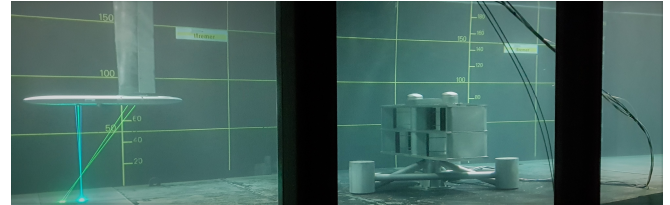
Fig. 1. Ducted 2-VATT in the Flood tide Configuration in the Ifremer wave and current tank, with the 3 Components LDV probe upstream.
