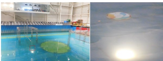
Fig. 9. The small-scale model in the wave tank
