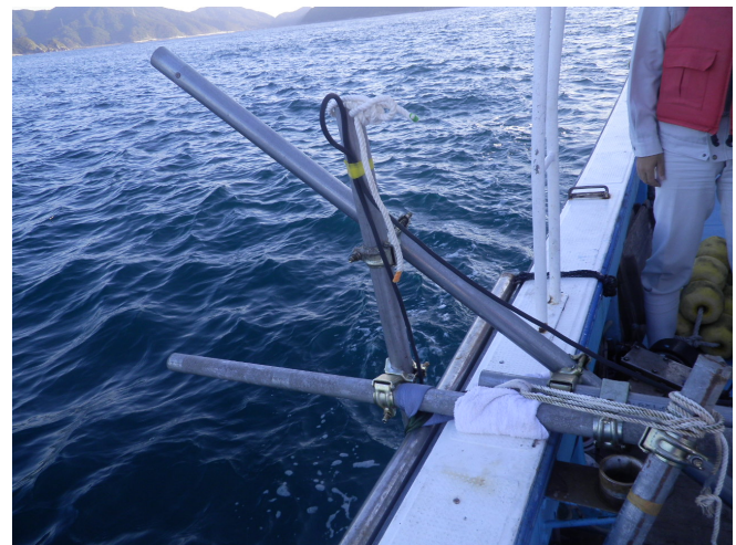
Fig. 5. ADCP-vessel attachment system.
