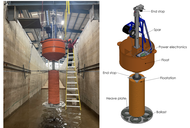
Fig. 1. LUPA WEC: picture (left) with a person for scale, and rendering (right, reproduced with permission from [6]) identifying main components.
