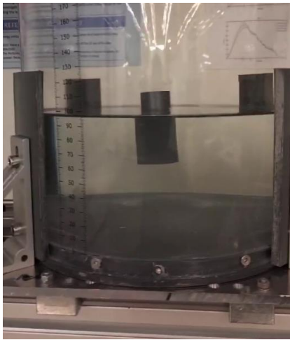
Fig. 6. First successful run of the Wavebox. A 3-cm wide cylinder is excited by the same surge-only excitation as in Fig. 5. After motor control adjustments, slosh excitation is minimal, and the cylinder has sufficient inertia that it exhibits an obvious phase difference with the water motion. The pure-surge excitation also led to a small pitch response, potentially providing a potentially interesting way to analyse coupling of surge and pitch for various shapes.
