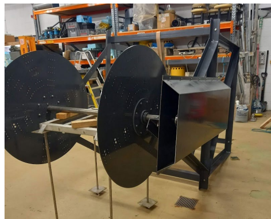
Fig 3. Partially assembled TACT at Queen's Marine Laboratory workshop, Portaferry with pulley guard attached.
