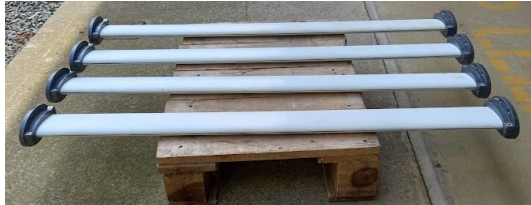
Fig 4. NACA0020 composite blades fitted with blade end clamps to attach to the end disks.
