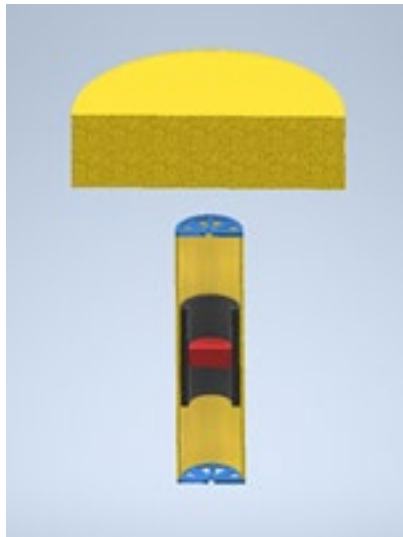
Fig. 1 Prototype of an IPS buoy wave energy converter being developed. The yellow parts oscillate, the red part is the translator of an electric generator, which is coupled to the water contained in the cylinder.
