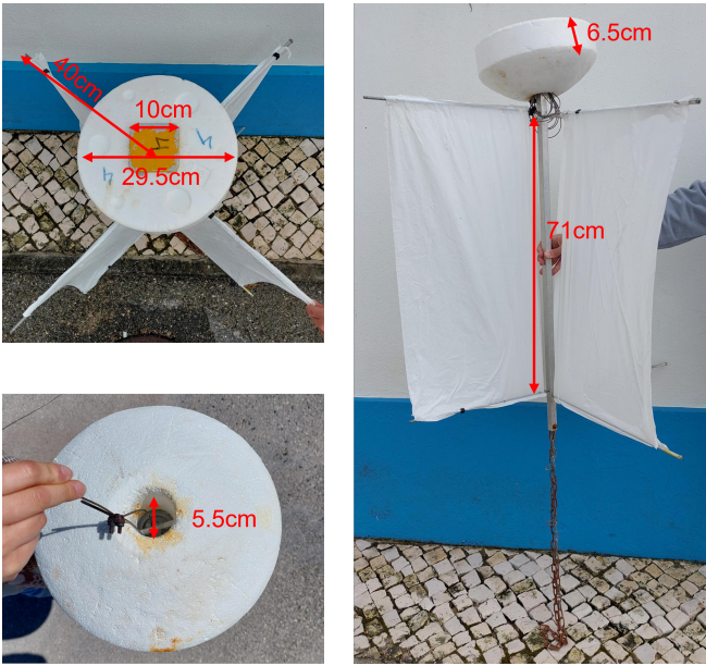
Fig. 4. Drifter design. Top left: top view. Bottom left: bottom of the float. Right: side view.
