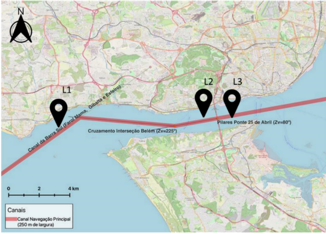
Fig. 3. Potential locations of tidal turbines in the Tagues River, the pink line representing the navigation channel.
