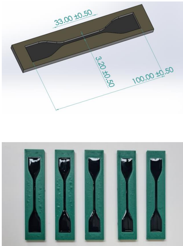
Fig. 2. Dimensions of the mould for tensile tests (unit: mm, samples thickness: 3 mm).
