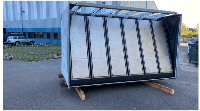
Fig. 11. Arrival of the elevated-hinge wave generator to the HWRL.
