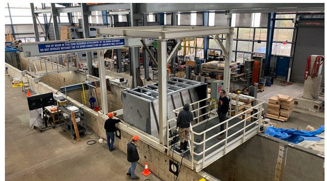
Fig. 13. Setting up and commissioning of the wave generator in the Large Wave Flume. Deployment at Bay 8 with the flume gantry crane.
