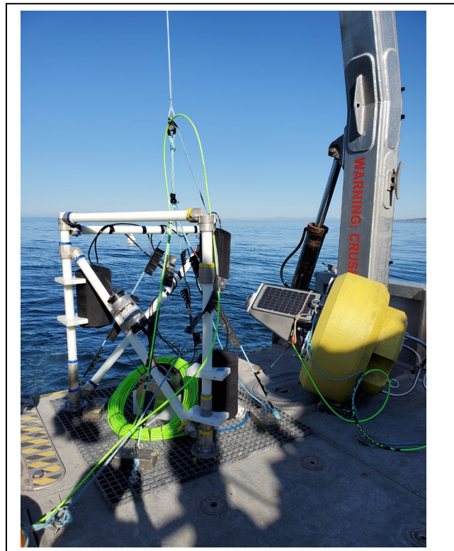
Fig. 2. The NoiseSpotter® consisting of three vector sensors housed inside the black cylindrical pods, along with surface telemetry buoy.
