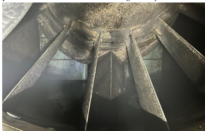
Fig. 4. Attachment of barnacles to wicket gates.
